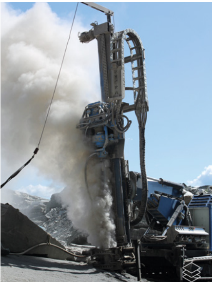
VD100 drilling in medium-hard rock, 100 m deep, hole diameter 135 mm, flushing with air.
